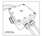
The LINK box is cast of aluminum and completely sealed to the environment. Each LINK box has two RJ45 connectors for INPUT/OUTPUT, as well as 4 cable glands to protect the connections with the Light Sprite Structures. The LINK can be slightly buried in the ground for visual purposes, as well as to avoid any hazards during the installation.
